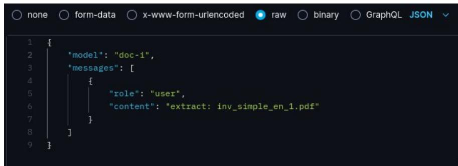
A screenshot of a browser's developer tools showing a JSON API request. The request is a POST to 'http://localhost:3001/api/document'. The 'raw' tab is selected, showing the following JSON payload:
